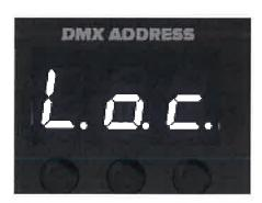
When the Pro Jet is receiveing DNOX the unit will enter a lockout state. Either removing DNOX or holding down a button for 5 seconds will allow readdressing.
