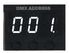
While addressing the Pro Jet, there is a 3 second window before the address is store. If the unit is receiving DMX it will re-enter its lockout state.
