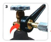
3. Position your CO<sub>2</sub> tank in a nearby location. Make sure the tank is stable, and won't tip over. Tanks should be secured with retcheting straps or chain to ensure they are secure.
