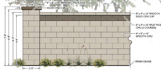
2 SECONDARY WALL Scale: 1/2" = 1'-0"
