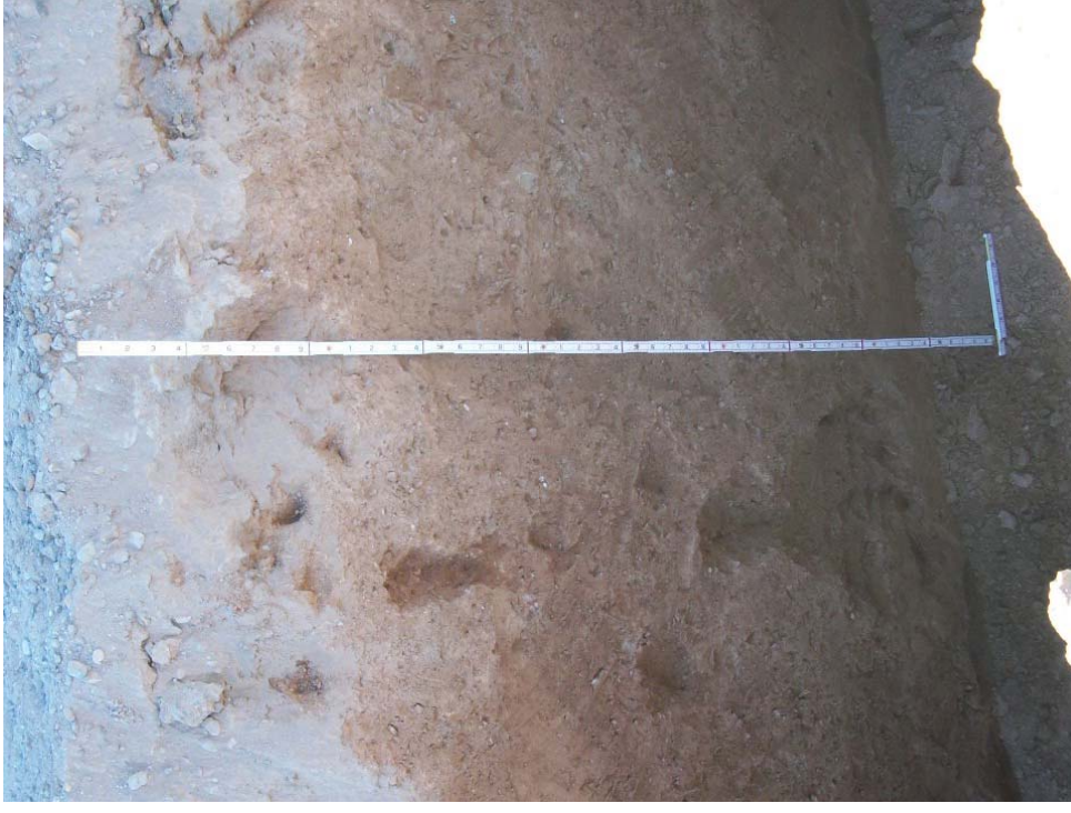
Photo 2: Soil profile in Trench RP-T4 sidewall. Dark yellow brown very dense sandy silt—silty sand with pea-sized gravel to 1' overlying porous sandy clay with pea-gravel lenses to 4.45' homogenous silt with minor fine sand, mottled with secondary caliche and filaments to 5'
