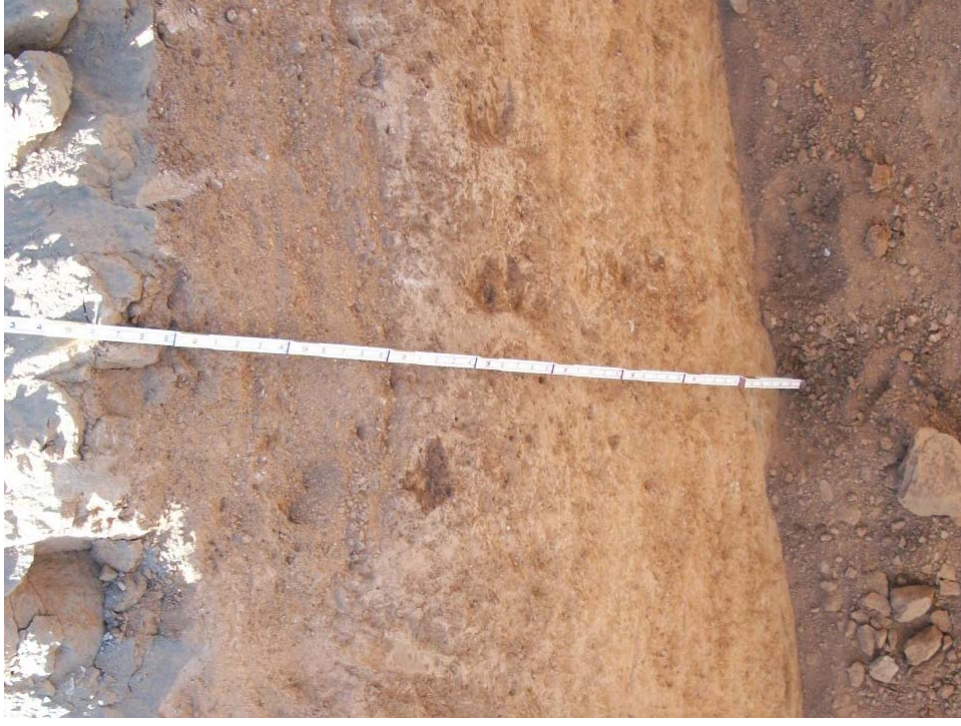
Photo 2: Soil profile in Trench RP-T2 sidewall. Dark orange-brown dense silty clay—clayey silt to 0.9' overlying poorly sorted stream channel deposits with fine to coarse sand and gravel to 1.75' overlying hard clayey silty with some sand, mottled with caliche, high shrinkage and expansion potential to 5'
