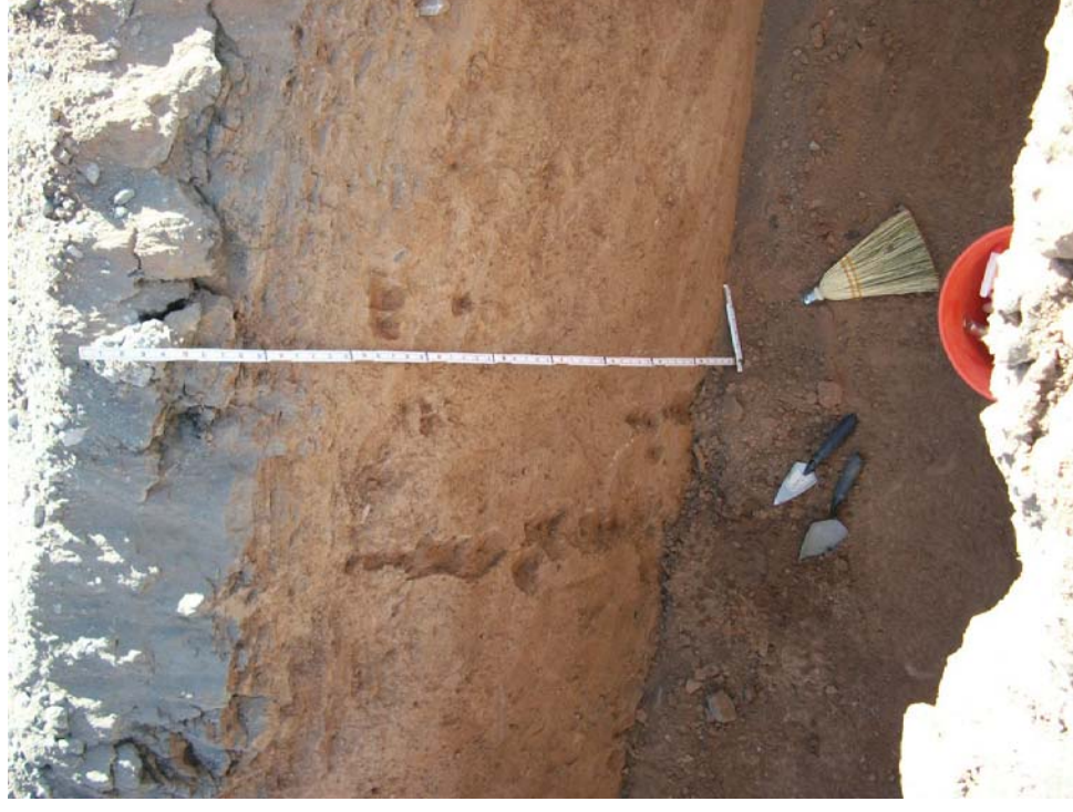
Photo 2: Soil profile in Trench RP-T3 sidewall. Coarse gravel with sand fill (ABC grade) to 0.68' overlying sheet flow deposit to 1.85' over yellow-brown porous medium dense to dense silty clay to 4.3' overlying light pink fine sandy clay with caliche nodules
