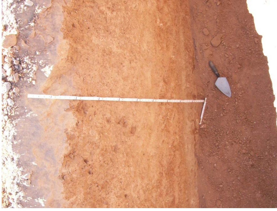
Photo 2: Soil profile in Trench RP-T1 sidewall. Orange-brown silty sand with gravel to 1.35' overlying dark yellow-brown silty clay to clayey sand with caliche filaments to 4.25' overlying silty clay with large caliche nodules to 5.2'. Very dense throughout.
