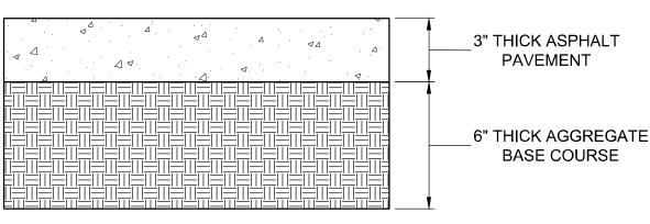
DRIVE-THRU STRUCTURAL SECTION DETAIL NOT TO SCALE
