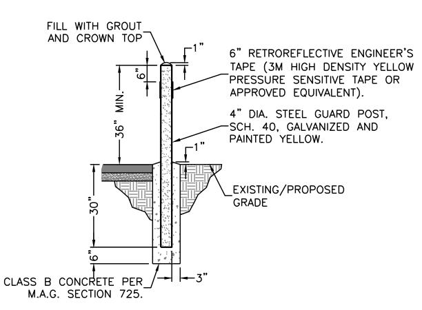
PAINTED STEEL BOLLARD DETAIL N.T.S.
