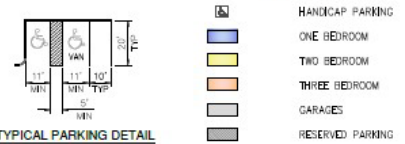
TYPICAL PARKING DETAIL NTS
