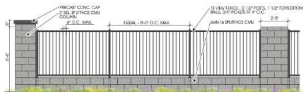
5 VIEW FENCE 'A' PLAN VIEW / ELEVATION NTS
