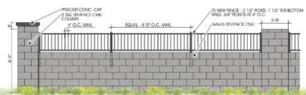
6 VIEW FENCE 'B' PLAN VIEW / ELEVATION NTS
