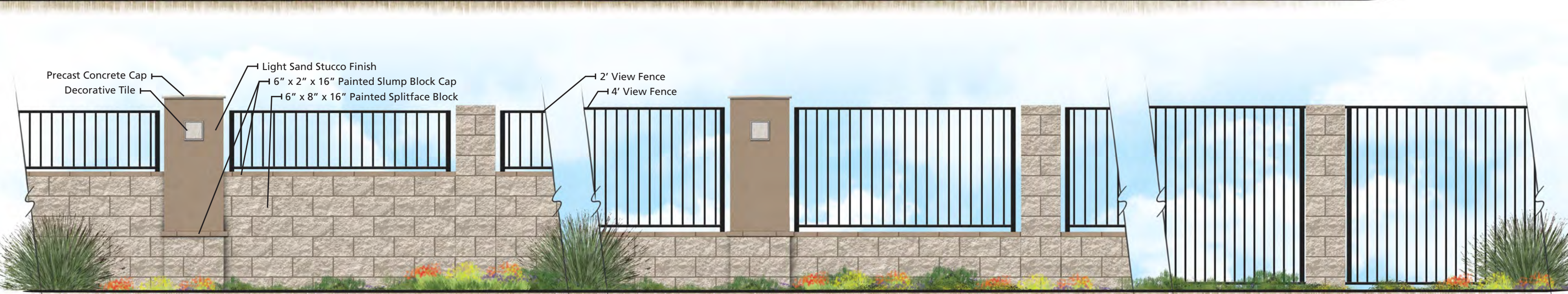
2' VIEW FENCE OVER 4' BLOCK WALL
