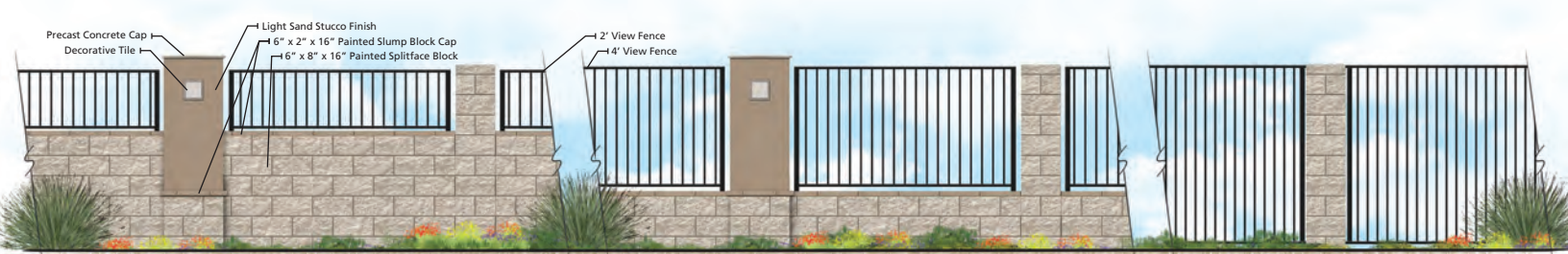
2' VIEW FENCE OVER 4' BLOCK WALL
